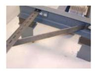
You support the vertical mounting angle with the provided support or in case of particularly high constructions, with the reinforcement strut "small" and the supporting angle.
