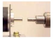
If the encoder is adjusted correctly, the flex coupling can be attached.
