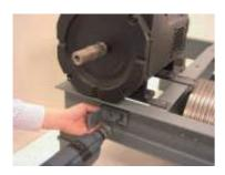
All following connections are made with the provided hexagon screws M10x30, if not described differently.
