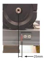
Mark the fixation holes at the supporting frame and drill at the marked points with a 10mm drill.
